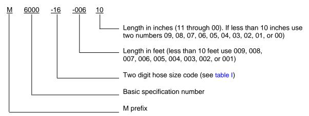
PIN example: M6000-16-00610 describes a 1-inch inside diameter hose that is 6 feet 10 inches long.
