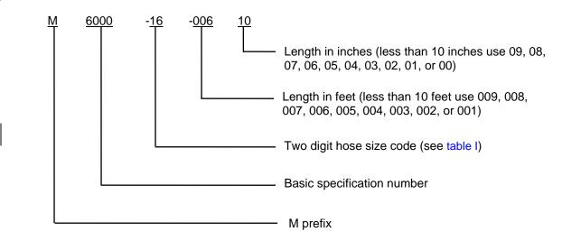
PIN example: M6000-16-00610 describes a 1-inch inside diameter hose that is 6 feet 10 inches long.
