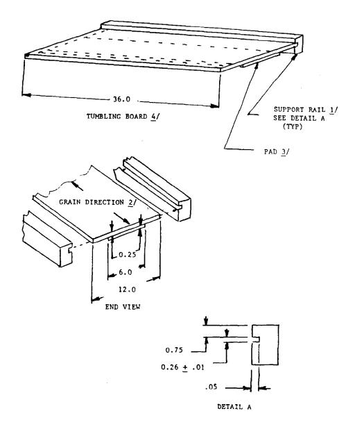
FIGURE 1. Projectile tumbling method
