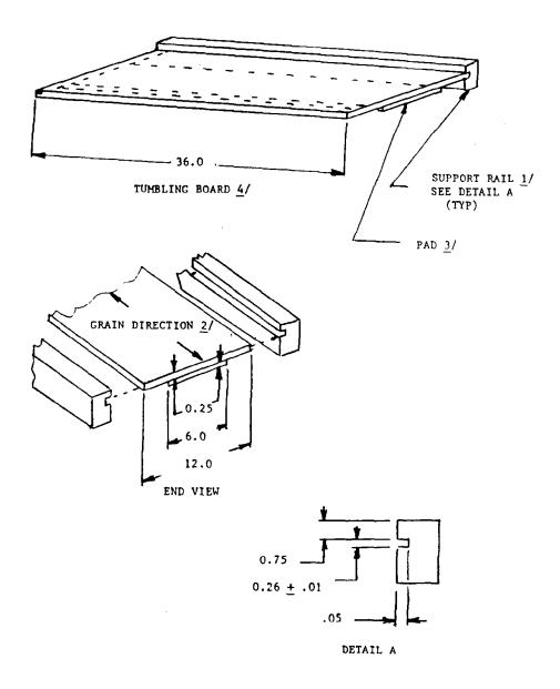
FIGURE 1. Projectile tumbling method
