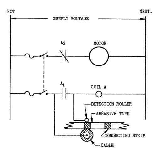
FIGURE 3. Schematic wiring diagram of abrasion tester.
