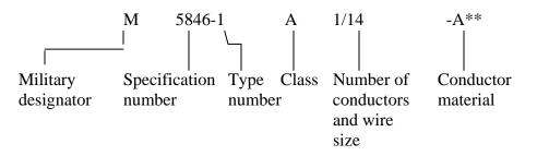
\*\* For single conductor wire the wire material shall follow the wire size preceded by a dash. A=Alumel. C=Chromel.
