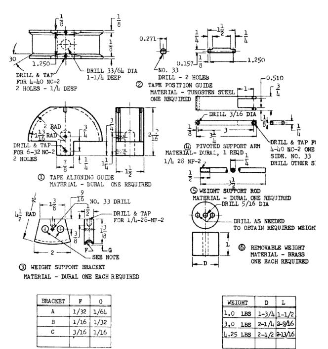
NOTE: WEIGHT OF BRACKET AND WEIGHT SUFPORT ROD TO BE 0.12 LBS. DRILL HOLES TO SUIT TO OBTAIN REQUIRED WEIGHT.
