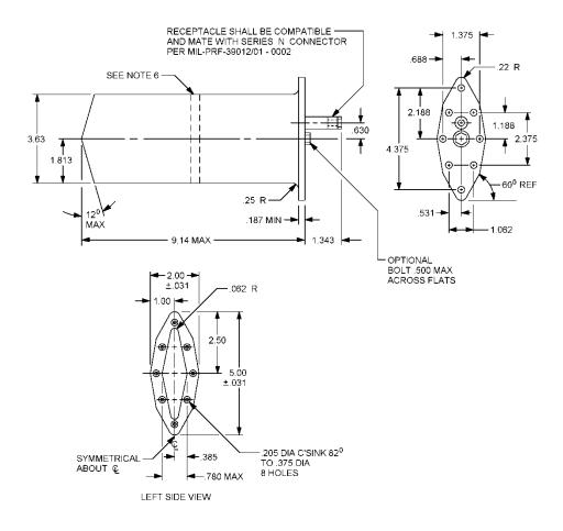
FIGURE 1. Dimensions and configuration.
