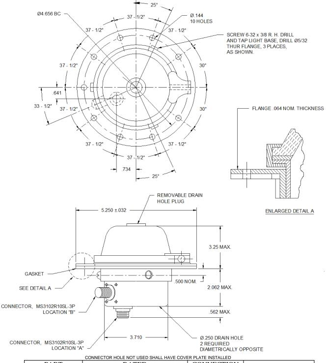
**PART RATED CONNECTION COVER COLOR VOLTS NUMBER WATTS LOCATION** M58085-1 28 DC 84 A **AVIATION RED** M58085-2 28 DC 84 В **AVIATION RED** M58085-3 28 DC 84 A or B **AVIATION RED**
