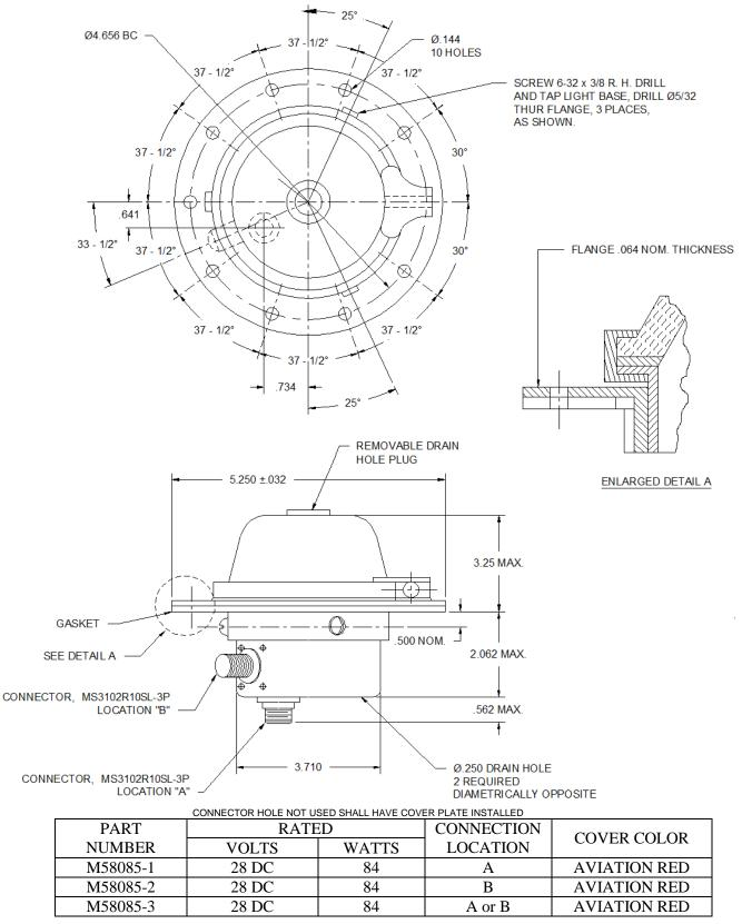
Dimensions in inches. Unless otherwise specified, tolerances, decimals  $\pm .016$ , angles  $\pm 1^{\circ}$ .
