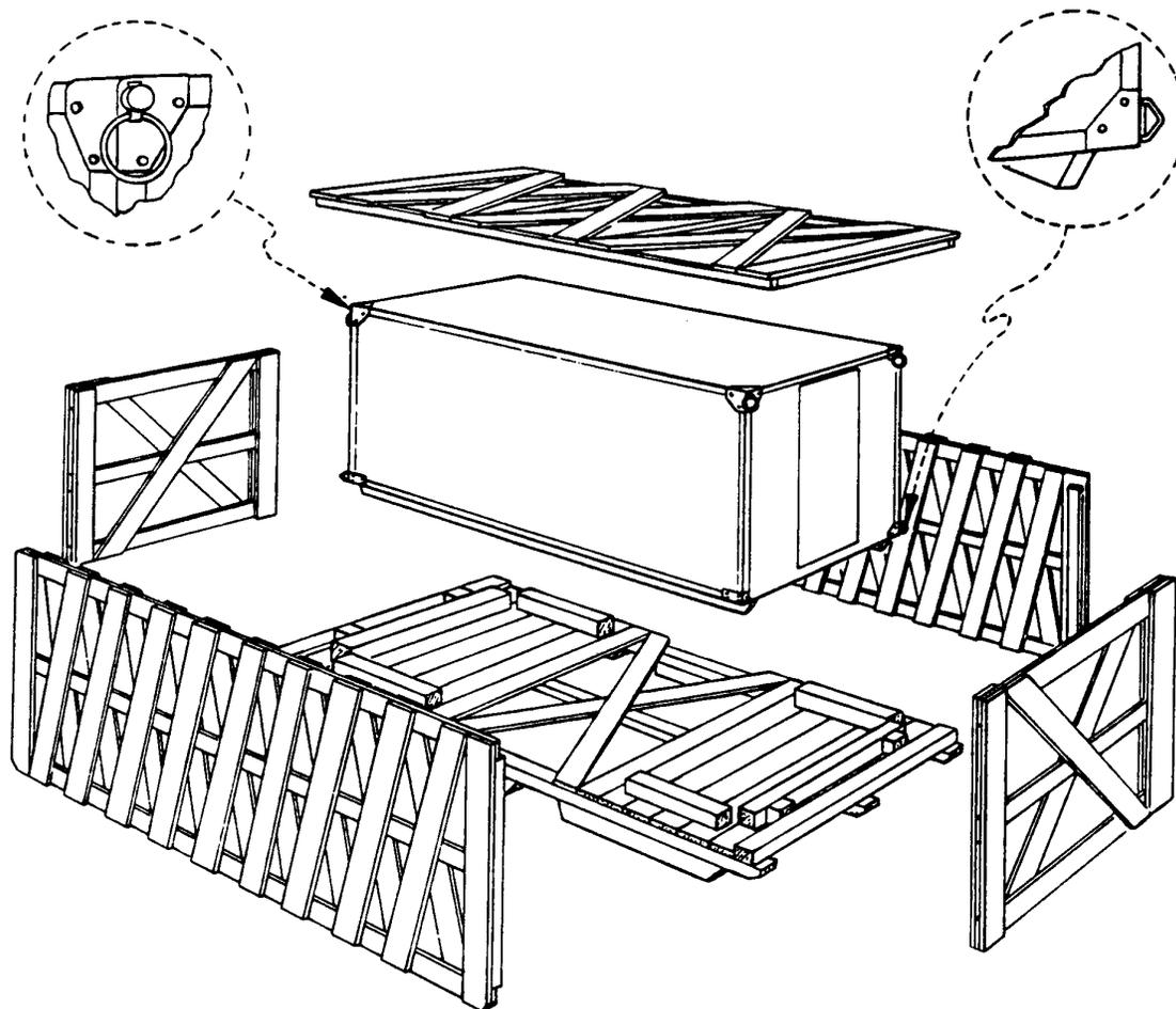
**NOTE:** Blocking at both ends of skid base is simulated to illustrate blocking requirements for shelters with projecting components.
