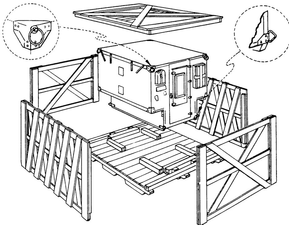
NOTE: Blocking at both ends of skid base is simulated to illustrate blocking requirements for shelters with projecting components.
