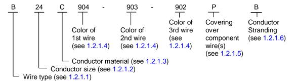
Type designation example: B24C904-903-902PB (MIL-DTL-16878/1 type wire; 24 AWG conductor size; copper material; 1st wire white base color, black first stripe, yellow second stripe; 2nd wire white base color, black first stripe, orange second stripe; 3rd wire white base color, black first stripe, red second stripe; covered with polyvinyl chloride jacket; 7 strands).
