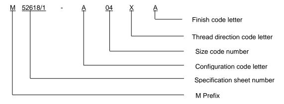
PIN example: M52618/1-A04XA indicates a 90° elbow for a 1/2 inch pipe, right hand threads, and finish is "as cast".
