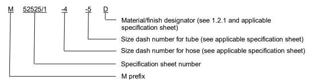
1.2.1 <u>Plating options</u>. To the users of this document, it is recommended that the use of carbon steel material with cadmium plating be used only when the other materials and finishes specified in this document cannot meet performance requirements.
