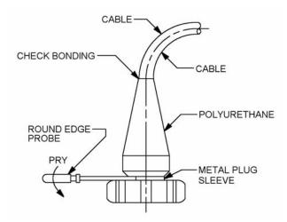
NOTE: Use round edge probe (rigid plastic or metal) with no sharp edges or corners, do not use screwdriver.
