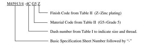
M45913/4-4CG5Z = Nut Self-Locking Hexagon, all-metal locking feature, .250-20 UNC-3B thread, Grade 5 steel, zinc plated.
