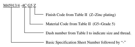
M45913/4-4CG5Z = Nut Self-Locking Hexagon, all-metal locking feature, .250-20 UNC-3B thread, Grade 5 steel, zinc plated.
