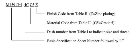
M45913/4-4CG5Z = Nut Self-Locking Hexagon, all-metal locking feature, .250-20 UNC-3B thread, Grade 5 steel, zinc plated.
