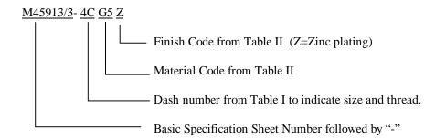
M45913/3-4CG5Z = Nut Self-Locking Hexagon, non-metallic locking feature, .250-20 UNC-3B thread, Grade 5 steel, zinc plated.
