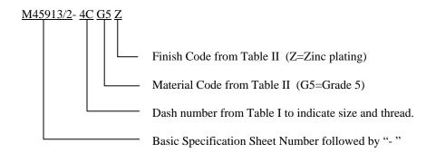
M45913/2-4CG5Z = Nut Self-Locking Hexagon, all-metal locking feature, .250-20 thread, Grade 5 steel, zinc plated.
