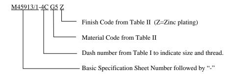
M45913/1-4CG5Z = Nut Self-Locking Hexagon, non-metallic locking feature, .250-20 thread, Grade 5 steel, zinc plated.
