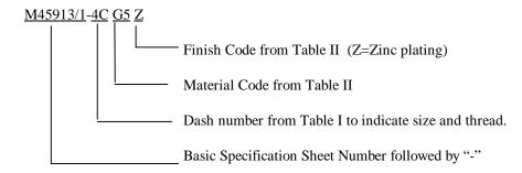
M45913/1-4CG5Z = Nut Self-Locking Hexagon, non-metallic locking feature, .250-20 thread, Grade 5 steel, zinc plated.
