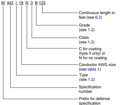
1.3 <u>Part or Identifying Number (PIN)</u>. The PIN to be used for cable acquired to the specification may be created as follows:
