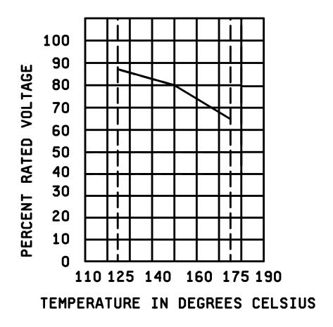
FIGURE 2. Voltage derating with temperature (125°C to 175°C) (styles CL10, CL13, CL14, CL16, CL17, and CL18 only).
