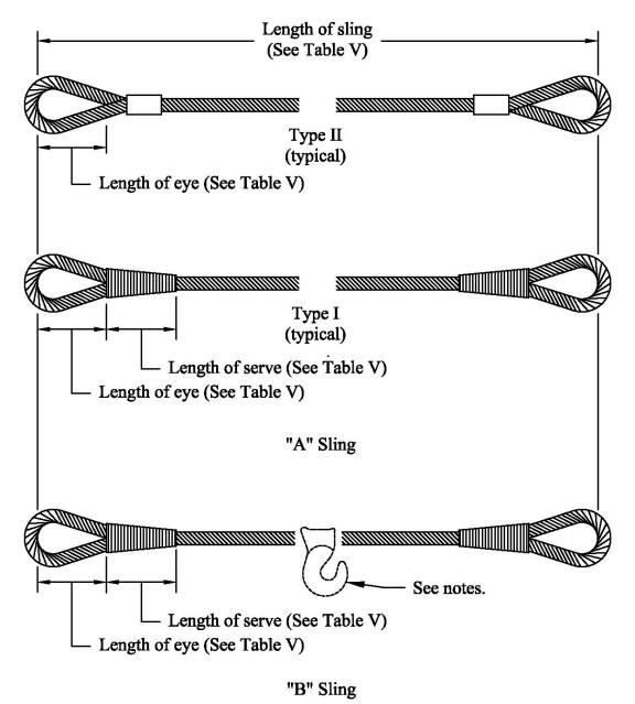
NOTES: 1. "B" sling is furnished with a choker hook. 2. Hook size shall match up with rope size.
