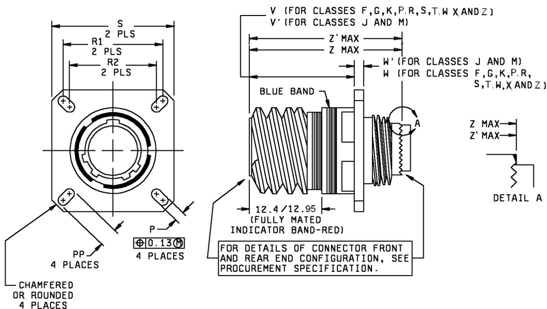
FIGURE 1. Receptacle, classes F, G, J, K, M, P, R, S, T, W, X and Z.
