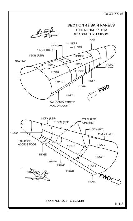
FIGURE 4. Example of a typical skin diagram.
