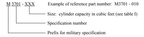
M3701 - 010 indicates a 10 ft<sup>3</sup> capacity cylinder, with an outer diameter of 4.0 inches  $\pm 0.5$  inch, a height of 12.5 inches  $\pm 1.0$  inch, 3/8-18NGT inlet threads, and a valve specified as AA59860-005
