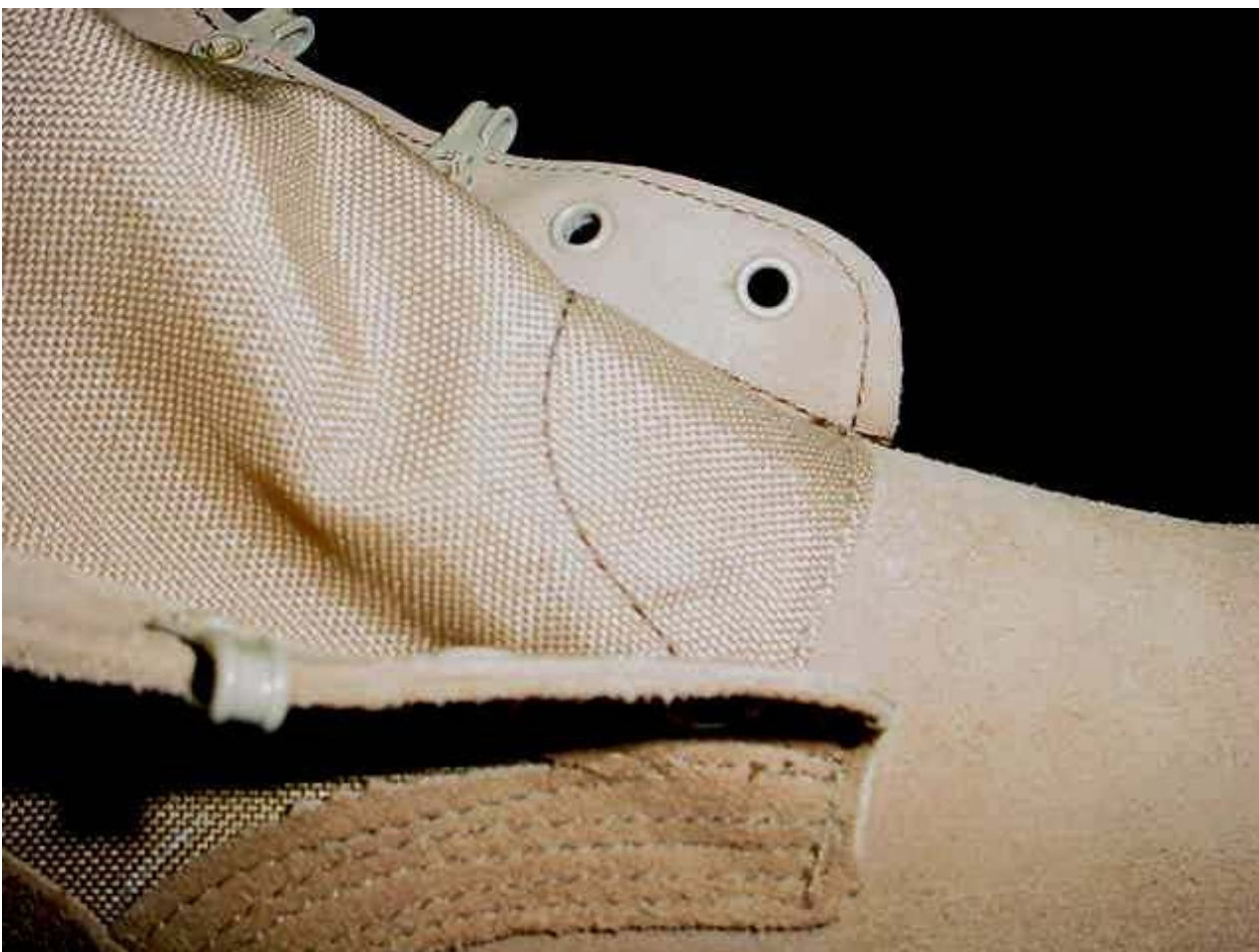
FIGURE 3B. Close up view of vamp/gusset seam (lateral view).
