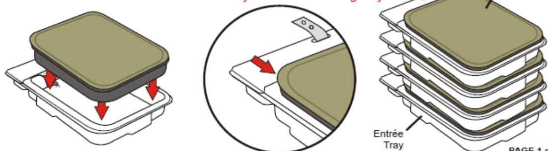
FIGURE 14. Assembly Instructions for Type I Heater Module
