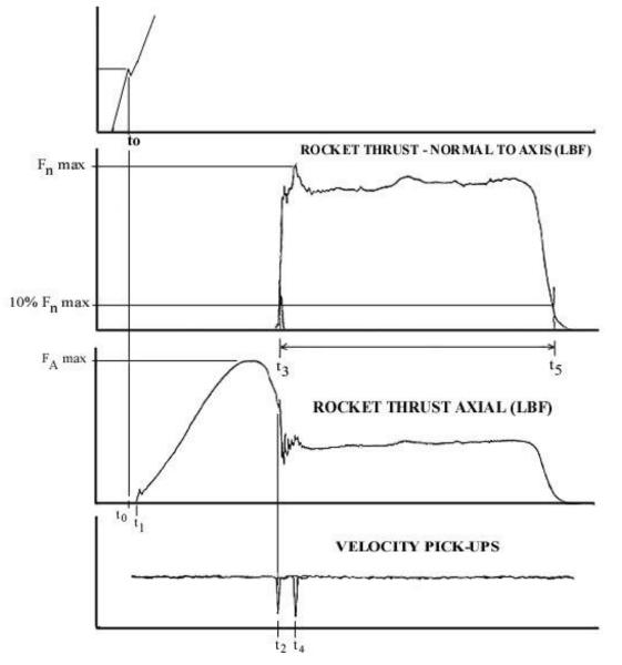
t<sub>1</sub> - t<sub>0</sub> = Catapult Ignition Delay Time
