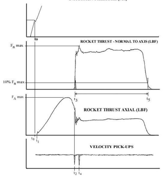
$t_1$  -  $t_0$  = Catapult Ignition Delay Time
