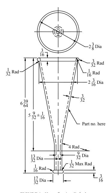
FIGURE 1. Horn, flyer's relief tube.
