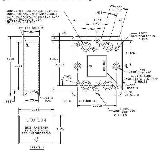
FIGURE 1. Outline and dimensions for mounting MT-1995/A.
