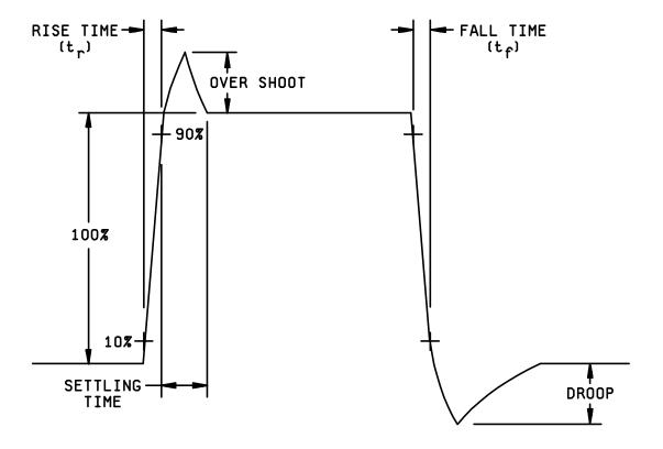
FIGURE 14. Pulse measurements.
