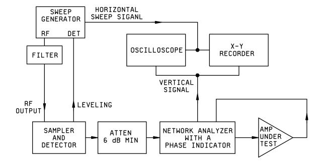
FIGURE 9. Phase linearity test setup.
