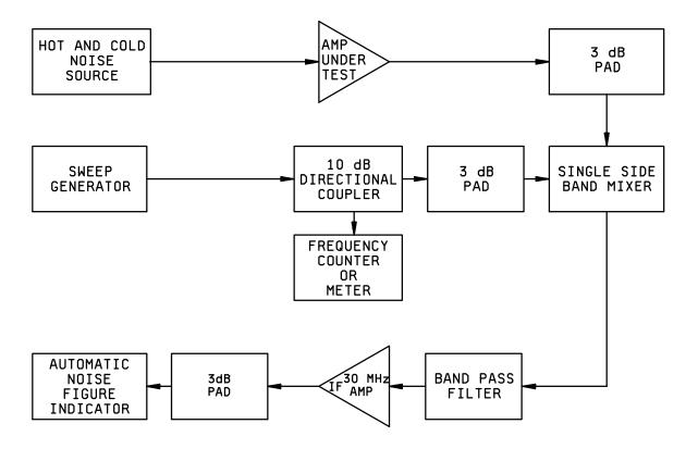
FIGURE 6. Low noise figure test setup.
