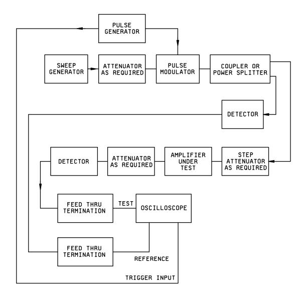
FIGURE 14B. Output pulse response test setup.
