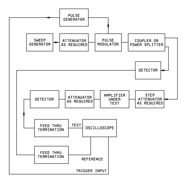
FIGURE 14B. Output pulse response test setup.
