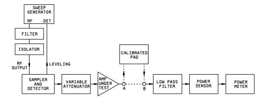
FIGURE 3. Output power test setup.
