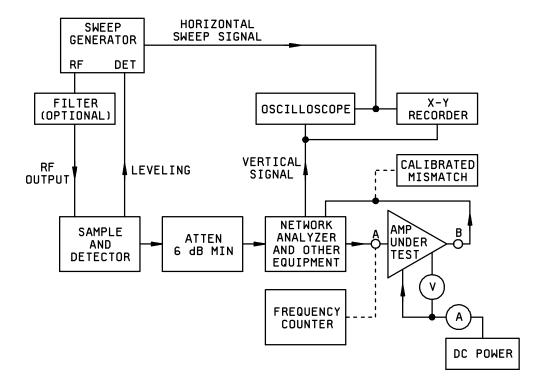
FIGURE 1. Gain, gain flatness and VSWR test setup.
