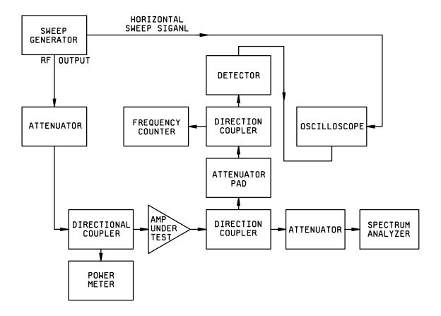
FIGURE 12. Harmonic and spurious test setup.
