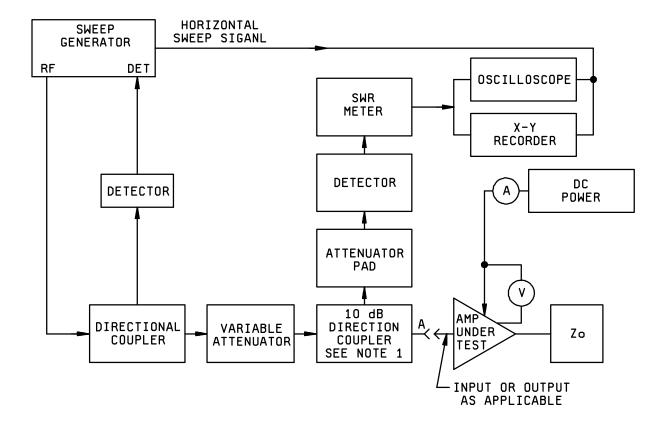
NOTE 1: The directivity of the directional coupler shall be such as to permit measurement of the VSWR with the appropriate accuracy.
