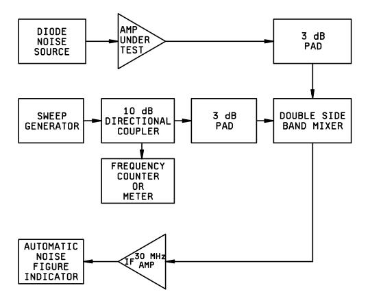
FIGURE 7. Noise figure > 3 dB test setup.
