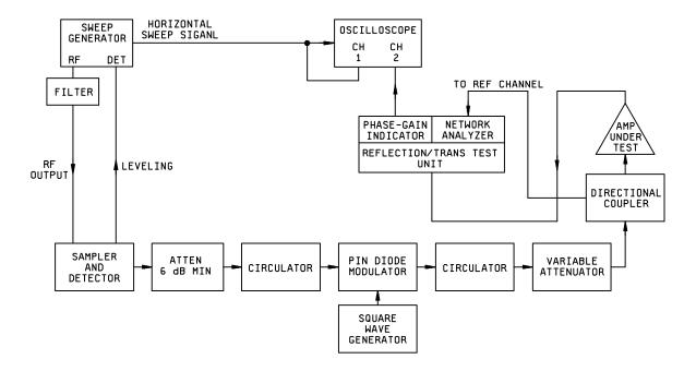
FIGURE 11. AM/PM conversion test setup.
