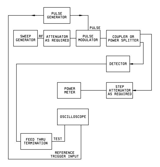
FIGURE 14A. Pulse response calibration setup.
