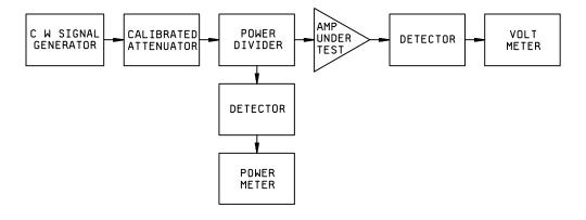
FIGURE 13. Logarithmic accuracy and sensitivity test setup.
