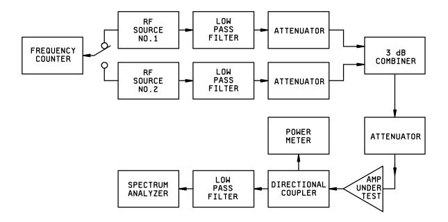
FIGURE 8. Intercept point test setup.
