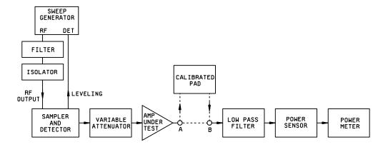
FIGURE 3. Output power test setup.
