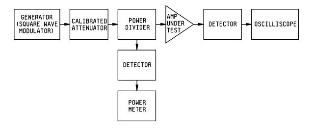
FIGURE 4. Video output test setup.
