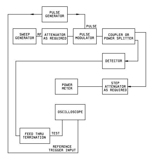
FIGURE 14A. Pulse response calibration setup.
