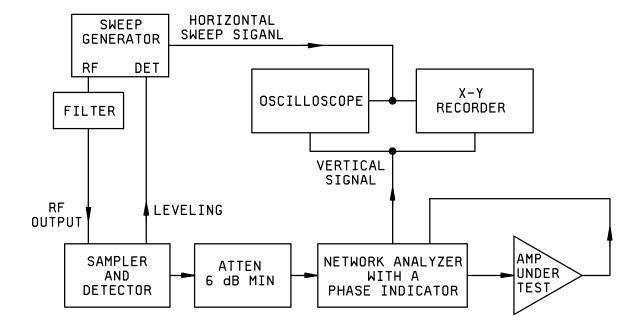
FIGURE 9. Phase linearity test setup.
