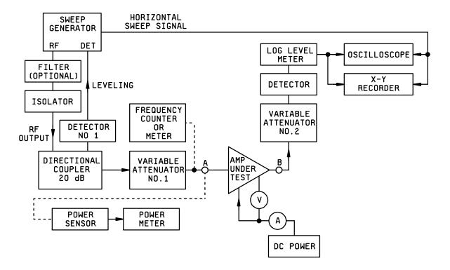
FIGURE 2. Gain and gain flatness test setup.
