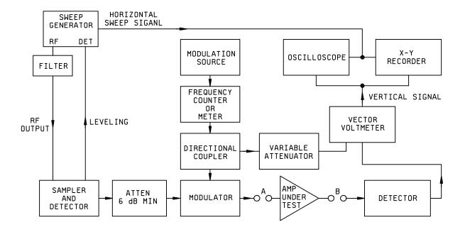
FIGURE 10. Group delay test setup.
