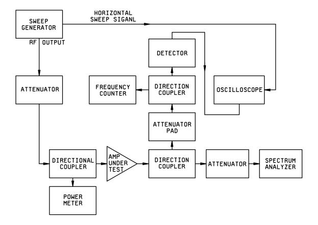
FIGURE 12. Harmonic and spurious test setup.
