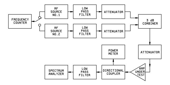
FIGURE 8. Intercept point test setup.
