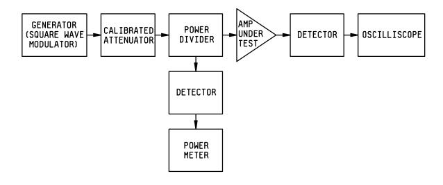
FIGURE 4. Video output test setup.
