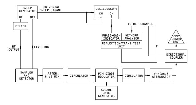
FIGURE 11. AM/PM conversion test setup.
