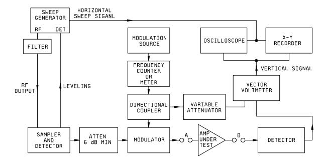
FIGURE 10. Group delay test setup.
