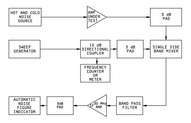
FIGURE 6. Low noise figure test setup.
