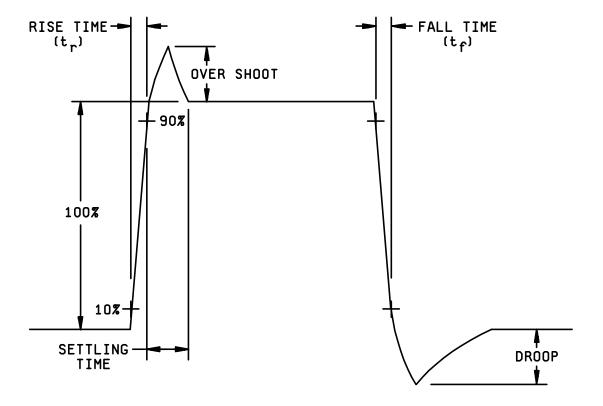
FIGURE 14. Pulse measurements.
