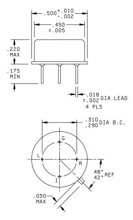
FIGURE 1. Outline drawing for mixers PIN M28837/9-01 through M28837/9-04.
