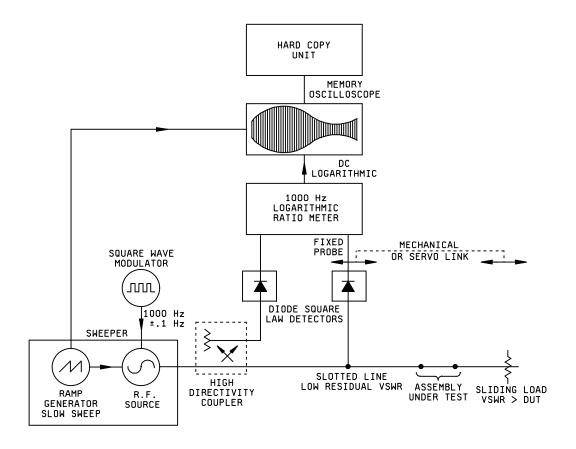
FIGURE 2. VSWR test using coupled sliding load.
