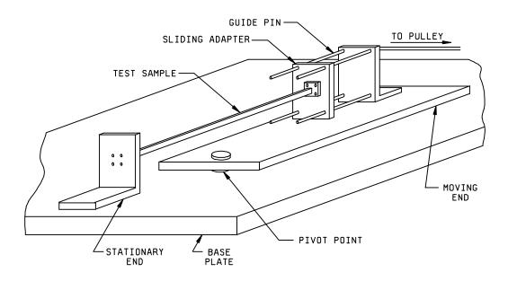
FIGURE 3. Flexure test figure.
