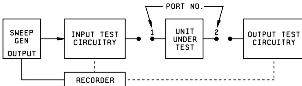
NOTE: The input and output circuitry shall be such that the errors in the measurement quantities are small. The values given in the specification sheet include worst case test circuitry errors.
