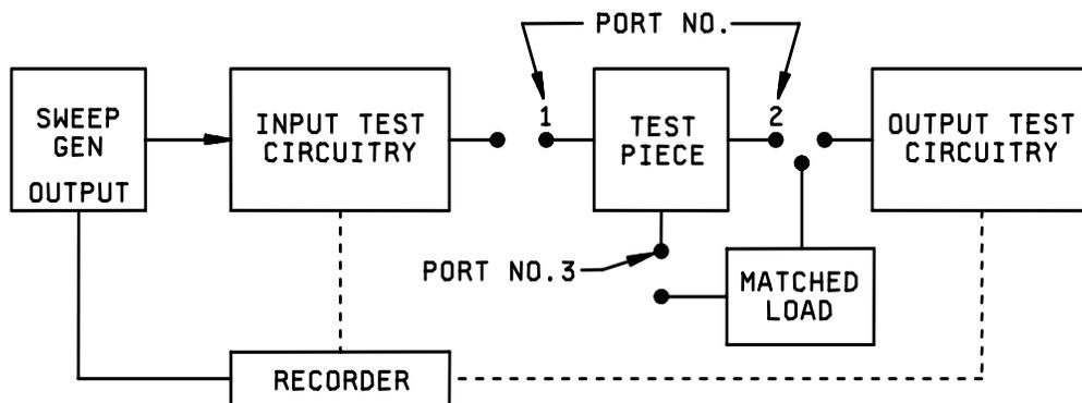
NOTE: The input and output circuitry shall be such that the errors in the measurement quantities are small.
