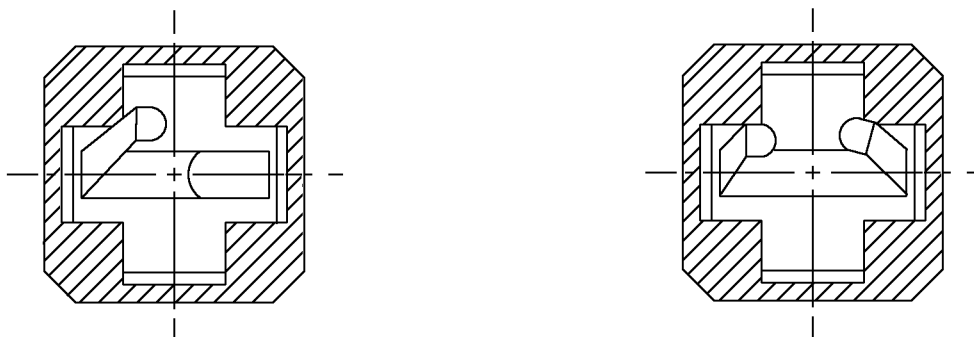
FIGURE 1D - Single contact line twisted.
