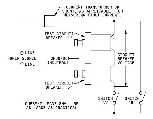
RUPTURE CURRENT SHALL BE MEASURED BY A CURRENT TRANSFORMER OR SHUNT AS INDICATED AND RECORDING OSCILLOGRAPH HAVING A RESPONSE TO AT LEAST 3000 HZ. THE VOLTAGE ACROSS THE BREAKERS INCLUDING THE TRANSIENT RECOVERY VOLTAGE AFTER THE INTERRUPTION OF CURRENT SHALL ALSO BE RECORDED.
