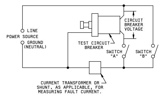
RUPTURE CURRENT SHALL BE MEASURED BY A CURRENT TRANSFORMER OR SHUNT AS INDICATED AND A RECORDING OSCILLOGRAPH HAVING A RESPONSE TO AT LEAST 3000 HZ. THE VOLTAGE ACROSS THE BREAKER INCLUDING THE TRANSIENT RECOVERY VOLTAGE AFTER THE INTERRUPTION OF CURRENT SHALL ALSO BE RECORDED.
