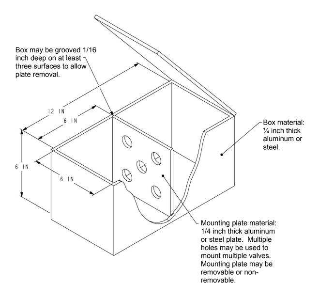
FIGURE 1. Container for rough handling test.
