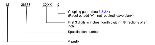
Example: M26633-9004A - 75 foot 1/2 inch length hose assembly with coupling guard.
