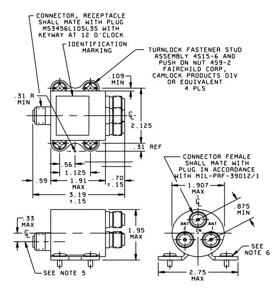
FIGURE 1. Outline and dimensions of switch type SA-521A/A.
