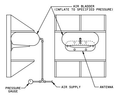
FIGURE 3. Static load test.
