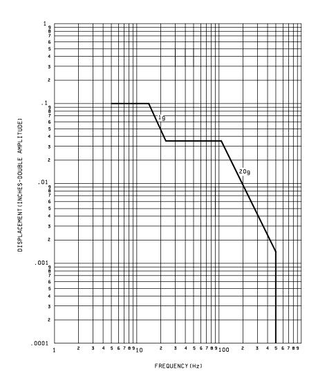
FIGURE 2. Vibration test curve.
