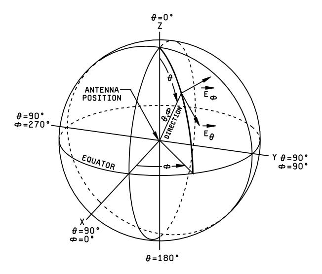
FIGURE 1. Standard spherical coordinate system used in antenna measurements.
