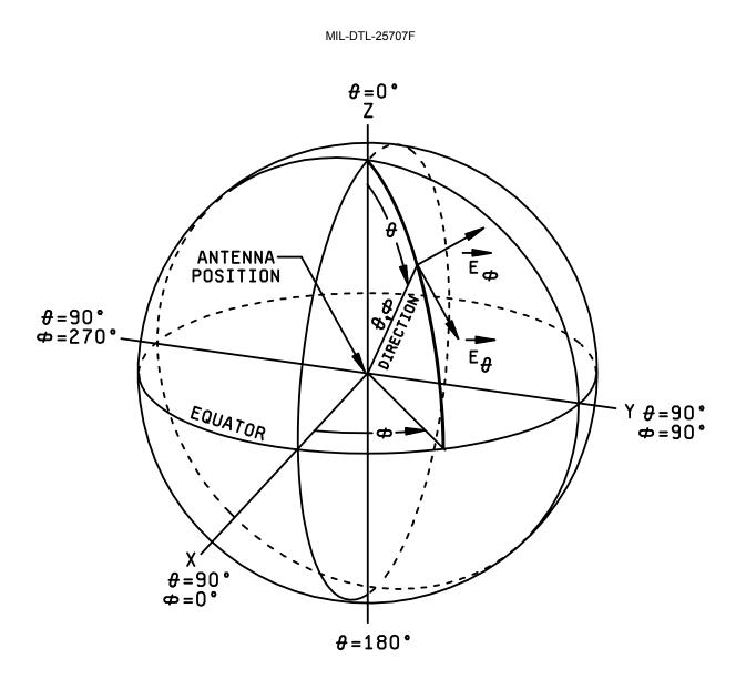
FIGURE 1. Standard spherical coordinate system used in antenna measurements.
