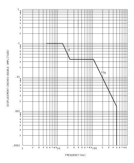
FIGURE 2. V bration test curve.
