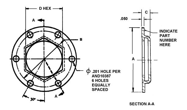
FIGURE 1. Flange coupling, dimensions, and configuration.
