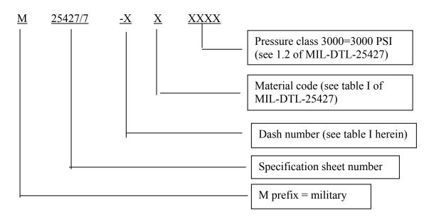
Example of part number: M25427/7-8C5000 represents 0.5 tube OD carbon steel coupling flange, 5000 PSI operating pressure
