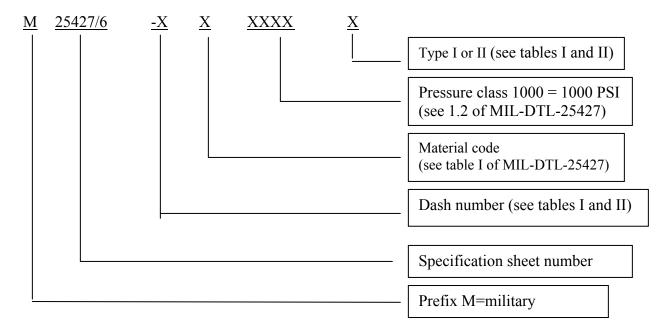
Example: M25427/6-8D1000 type II means 0.5 inch tube OD aluminum alloy coupling nut 1000 PSI operating pressure, type II.
