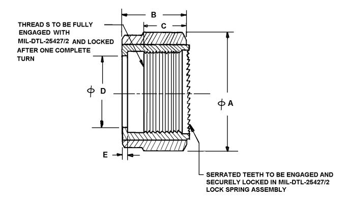
FIGURE 1. Coupling nut, dimensions and configuration for type I and II.
