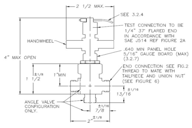
NOTE: TEST CONNECTION CAP SHALL BE SUITABLY DRILLED 1/16 DIA FOR VENTING.
