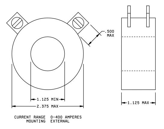
FIGURE 2. Outline dimensions for monitor current sensing transformer.
