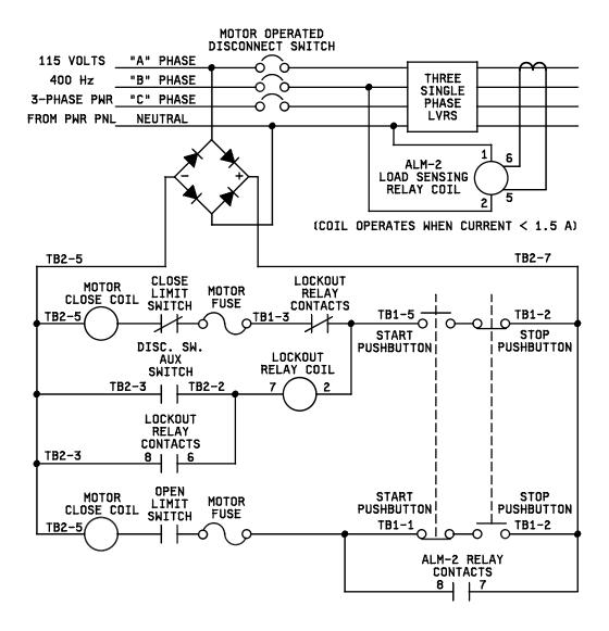
Typical wiring shown for monitor when connected to a circuit breaker with motor operator on a 115 volt circuit. Monitor normally open static contact is rated at a minimum of 10 amperes continuous, and intermittent rating of 15 amperes.
