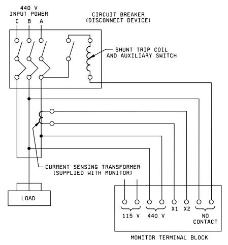
Typical wiring shown for monitor when connected to a circuit breaker with shunt trip coil on a 440 volt circuit. Monitor normally open static contact is rated at a minimum of 10 amperes continuous, and intermittent rating of 15 amperes.
