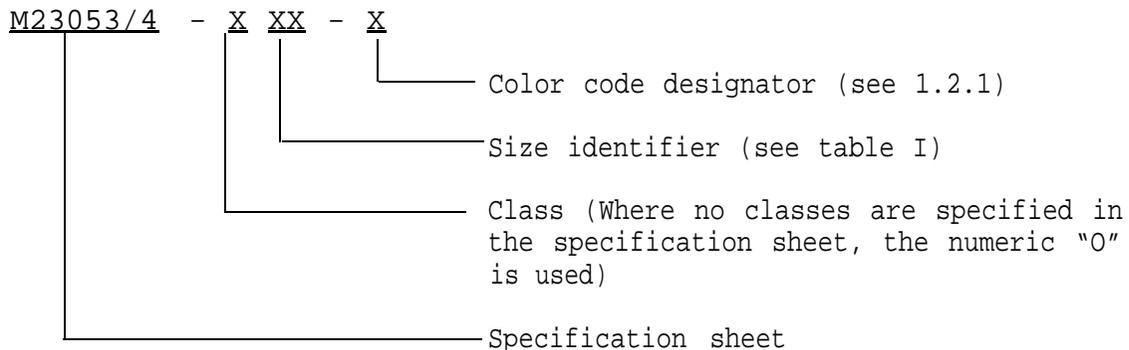
Example: Class 1, black sleeving .750 inch (19.1 mm) as supplied ID sleeving shall be identified as M23053/4-106-0.
