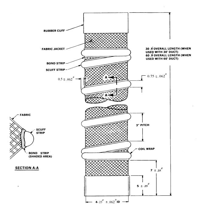
FIGURE 1. Duct assembly with scuff cover.
