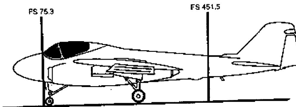
FIGURE 1. Crash handling structural hardpoints.
