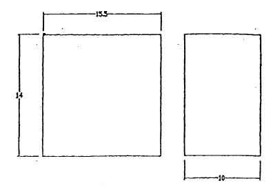
FIGURE 2. Basic PLC installation envelope.
