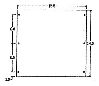
FIGURE 3. Basic PLC mounting footprint.
