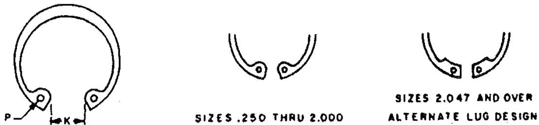
FIGURE 1. Type I, Class 1 Retaining Rings.
